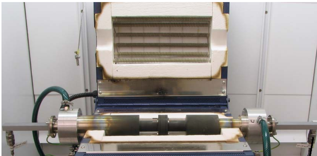
Figure 3: The figure shows the clam shell tube oven and the X-band waveguide contained in the hood. Note the cylindrical water jackets for cooling that are attached to the parts of the waveguide that are extending outside the oven.
